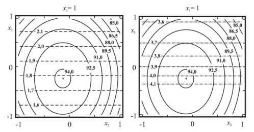
Fig. 3. Two-dimensional sections of the response surface characterizing the influence of the mixing time (x1), the rotation direction of the mixer auger shaft (x2) and the amount of material in the mixer hopper (x3) on the: a) finished product homogeneity coefficient vn (----y1), throughput capacity of the mixer Q(----y3); b) finished product homogeneity coefficient vn (-----y2)
