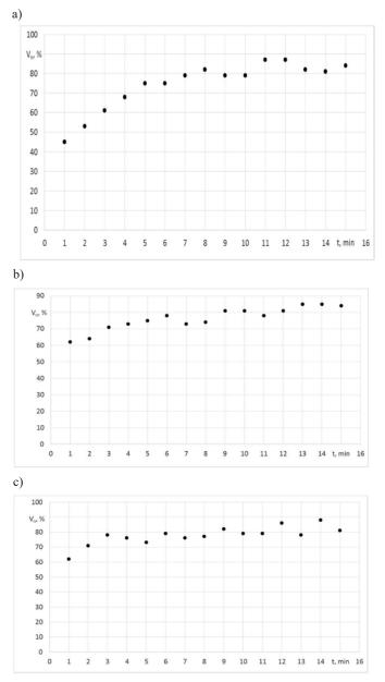
Fig. 1. Dependencies of the finished product homogeneity coefficient on the auger rotation time: a) forward, b) backward, c) forwardand-backward
